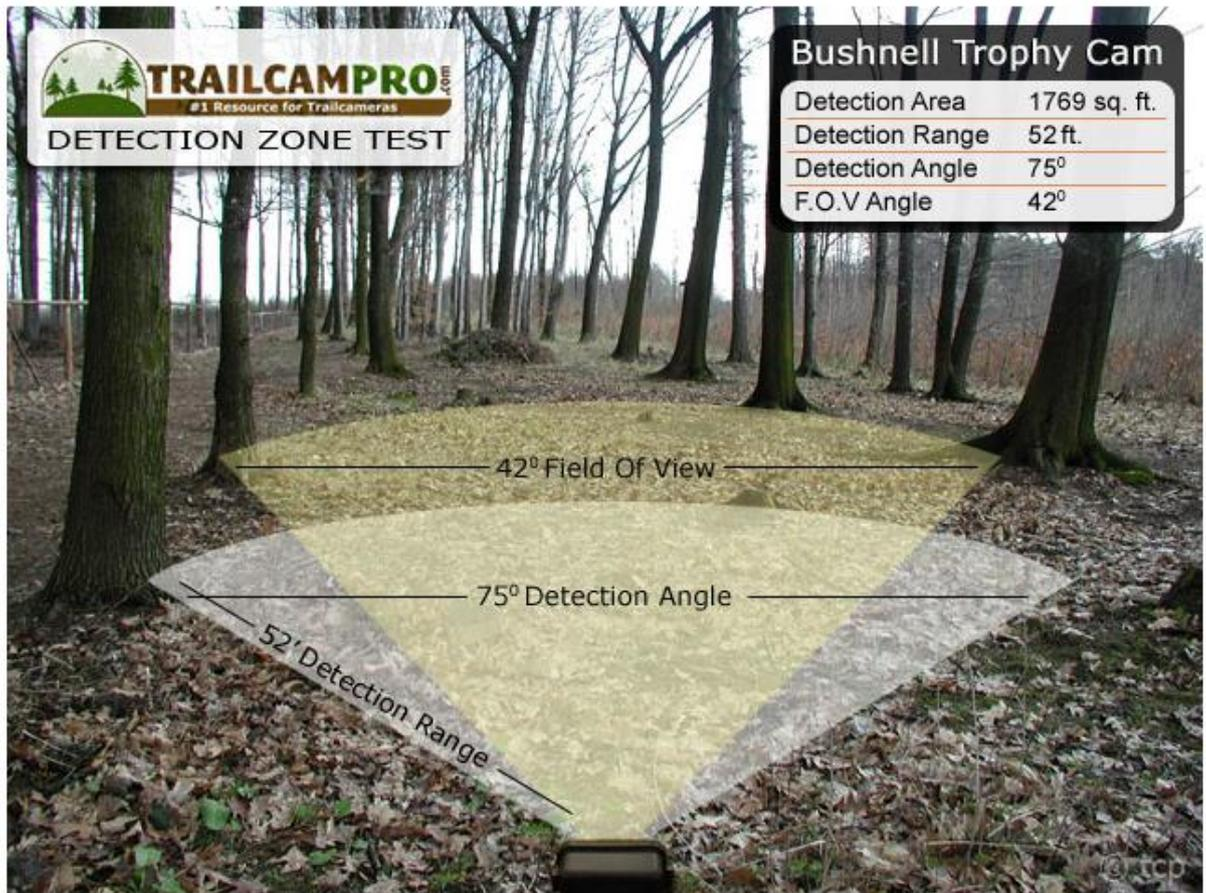
Figure 7: A comparison between detection area and field of view for a Bushnell Trophy camera trap.
